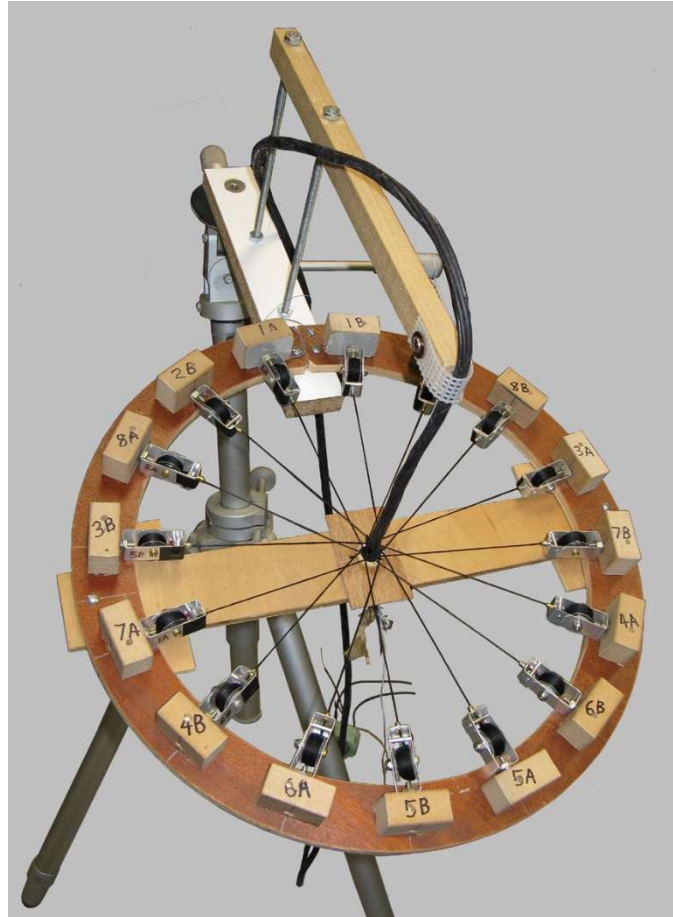
Figure 3 - Sturdy camera tripod holds braiding fixture in a comfortable position.
