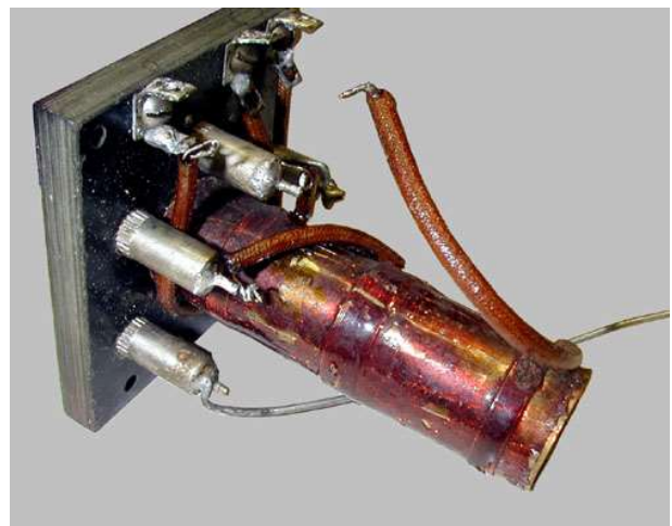
Unusual 3 section capacitor using copper windings for plates.
