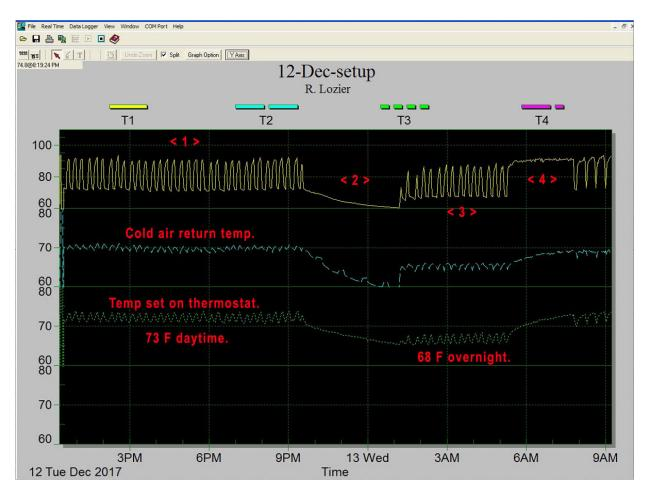
T1 = Measurement at a hot air register. T2 = Cold air return. T3 = Room temp.
