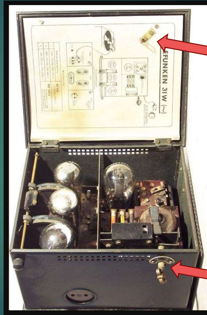
Lid is locked unless key switch is OFF. Won't turn ON unless lid is closed.
