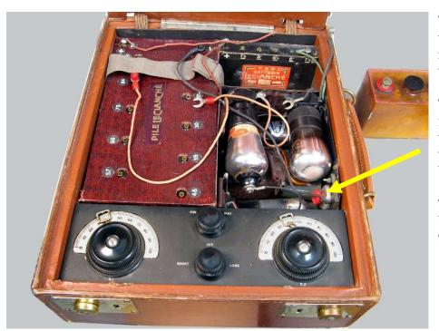
Two valves are mounted vertical in this picture, the other two valves are mounted at right angles underneath the two visible valves.
