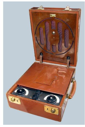
The receiver on exhibit here features a screen grid RF amplifier valve that was not in general use until 1929. There is a reaction (regenerative) detector and two stages of transformer coupled audio amplification.
