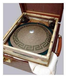
The two band frame antenna surrounds the pin driver high impedance loudspeaker.
