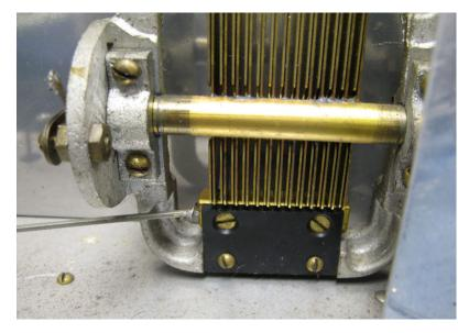
Here the unique mechanical approach to fine adjustment of this first tuned stage is made by a lateral shifting of the that shaft mounts the plates that rotor such they are more or less between the centered fixed stator plates of the
