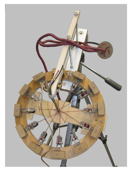
I engineered a braiding fixture with 16 shuttles. just like this 12 shuttle fixture I made for my Radiola M55 project, to permit braiding a jacket over a bundle of 9 wires (plus a filler strand of string); jute the filler necessarv to form а smooth, slightly oval cable.
