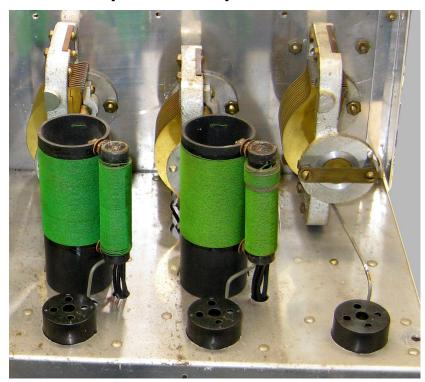
At left are the first and second RF amplifier transformers. The small coil is in the cathode circuit and the larger coil is the grid circuit.
