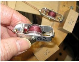
Once the bundle of wires are gathered parallel into alignment and secured by a spiral wrap of thread, it can be into braiding placed the fixture. In this case, about 36" of the bundle needs to have the braided jacket. To do the braiding takes about 8 hours work but the results are quite good. Good enough such that viewers are not likely to spend time questioning if the cable is not just 'new old stock' cable of the correct style.
