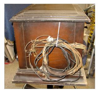
The battery cable is a little shorter than I would have expected. But there is evidence that the cable was never longer because each wire has a metal ID tag attached just about where you would expect it to be. There are 7 - 20 gauge wires and 2 - 16 gauge wires to service the filaments of the 8 type 01-A tubes.
