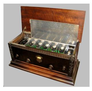
This, apparently, final design recognizes the industry trend to sell the notion of 'single dial tuning'. Sure enough all six tuning capacitors are ganged via large cut brass gears with a clever zerobacklash spring loading feature.
