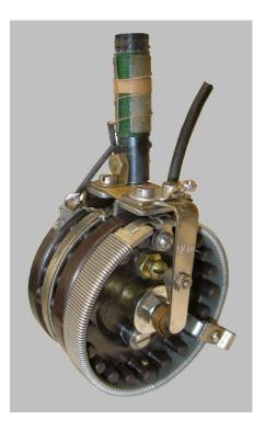
The only other repair was to the ingenious regeneration rheostat assembly. There was sinale of the cracked connection а resistance wire right at the termination of the wire. Gaining access for repair proved quite a challenge. With this write-up there is a copy of the July 2017 Radio Age description fascinating of this implementation of regeneration.
