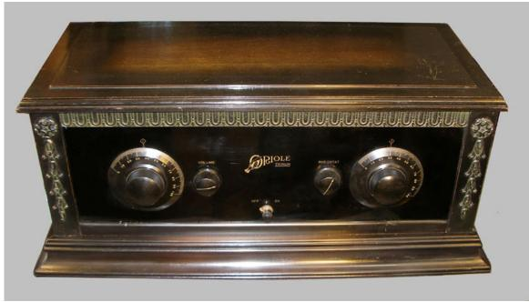
The middle series of 5 tube radios made by W-K Electric Co. incorporating cathode follower RF amplifiers. This model had only one competitor using this technology, the newly introduced '*Cascade*' by the Nunn – Landon Co. of Milwaukee, Wis. W-K's Anthony Winther held a patent on the cathode follower RF amplifier circuit. Did Nunn – Landon steal the technology? Historians have yet to uncover a definitive answer.
