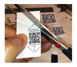
Tag is bonded to pre-painted aluminum sheet and cut out with heavy scissors.
