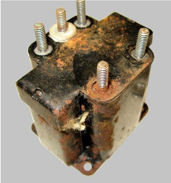
Figure 1- Rusted case requiring repaint but actual windings are still OK.
