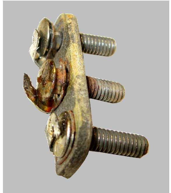
Figure 2 - Solder lug disconnected by rusting of #8 stud.
