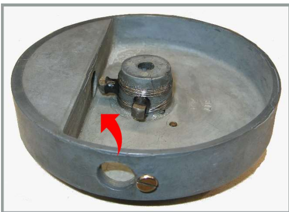
Figure 4 - Drum incorporates counterbalance weight; would have to be a separate lead part mounted inside a 3D printed plastic version.
