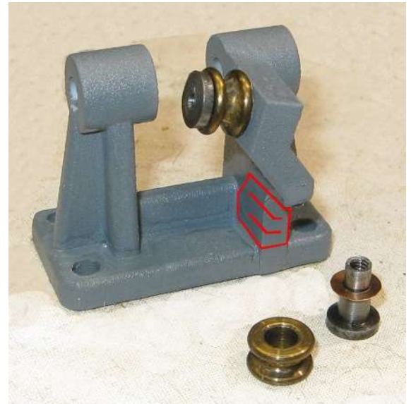
Figure 3 - Extra fill added for rigidity.
