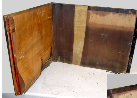
Both inside plies loose.
