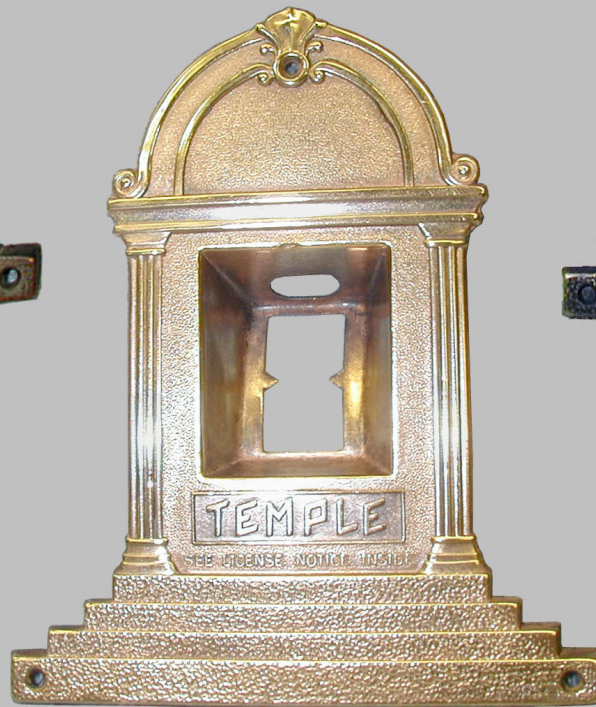
Part cleaned and highlight areas polished smooth.
