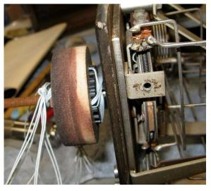
surfaces and wiped-away evidence of where the knob was sticking. The key thing for me was that the MDF and Kevlar cord were not abrasive enough to harm the Bakelite knob in any way.
