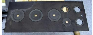
should you apply any water-based cleaners to old hard rubber. If there is any grime to remove, use a *waterless* hand cleaner like *Goop* or *Go-Jo*. Wipe-down with mineral spirits. If the surface is rough, sand with 220 grit paper lubricated with mineral spirits. To achieve a satin finish, continue rubbing with #0000 steel wool lubricated with spirits and using long linear strokes.
