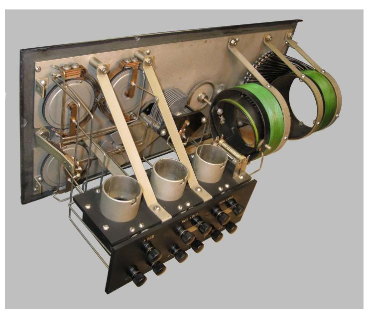
Note that the rheostats are equipped with an integrated switching scheme to route the audio output to a single phone jack regardless of whether you have headphones you want to connect to just the detector output or detector plus one stage of audio or wish to drive a loudspeaker from the second audio amplifier stage.
